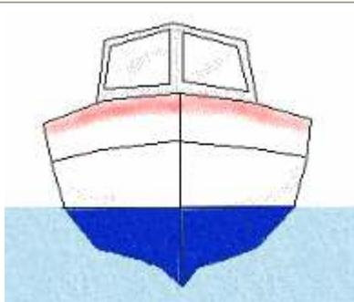
**Round bottom boat** - These move easily through the water, especially at slow speeds. They do, however, tend to roll unless they are outfitted with a deep keel or stabilizers. Many trawlers, canoes and sailboats have round bottoms.
