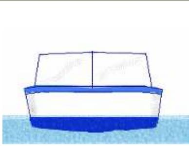
**Flat bottom boat** - These boats are generally less expensive to build and have a shallow draft (the part of the boat that's under the water). They can get up on plane easily but unless the water is very calm they tend to give a rough ride because of the flat bottom pounding on each wave. They also tend to be less stable and require careful balancing of cargo and crew. Examples of flat bottom boats might be Jon boats, small utility boats, and some high speed runabouts.
