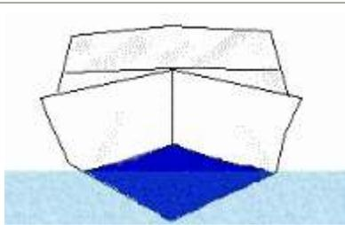
**Vee bottom boat** - The vee bottom tends to have a sharper entry into the water which provides for a smoother ride in rough water. They do, however, require more power to achieve the same speed. Many runabouts use the vee-bottom design.
