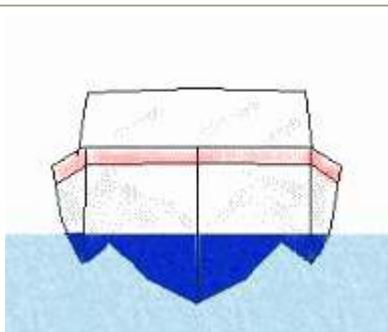
**Multi-hull boat** - Catamarans, pontoon boats and some house boats use a multi-hull design. The wide stance provides greater stability. Each of the hulls may carry any of the above bottom designs.
