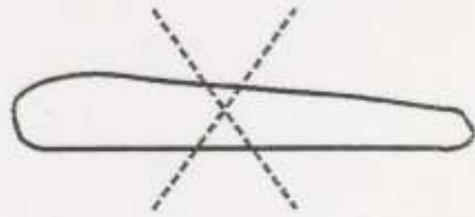
This airfoil (wing) shape is not correct. It will not furnish adequate lift. The plane will not glide at slow speeds.
