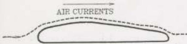
The air currents hug the air foil. The air speed is much greater above the wing than below the wing, thus resulting in proper lift.
